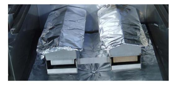
Line the bottom of the smoker with foil and punch a hole in the foil through the drain hole (always be sure the drippings can drain out). A clogged drain could cause grease to accumulate on the smoker floor, which could cause a fire.
